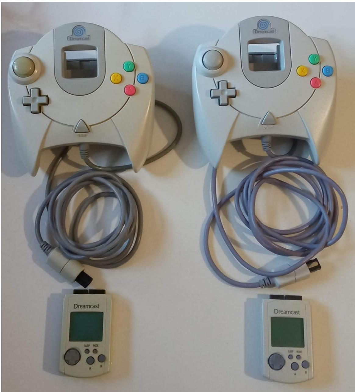
Figure 2. Difference in the ageing process of two Dreamcast Controllers and VMUs (PAL). Left has sustained heavy use since its release in 1999 and shows signs of yellowing in the casings and cables, and wear of the overall surface (specially visible on the stick); right has seen significantly less manipulation and exposure to UV radiation, retaining most of the original coloring.
